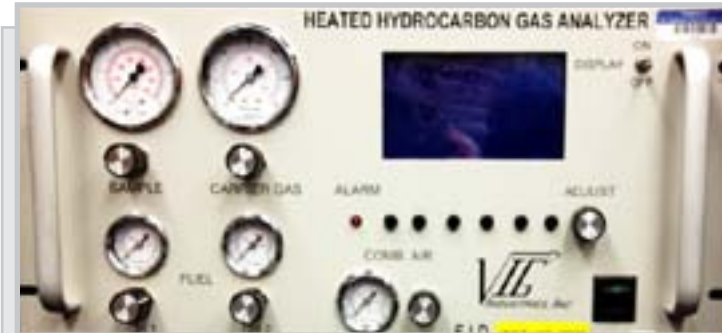
Air Hygiene utilizes a VIG 210 VOC analyzer that incorporates the Method 25A and Method 18 technologies into a single analyzer. Includes a built in gas chromatograph providing data for methane, ethane, VOCs, and total hydrocarbons.
