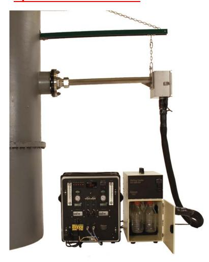
Ohio Lumex: RA915+ Analyzer with RP-91 Attachment for Ontario Hydro or 30b sorbent trap analysis on-site
